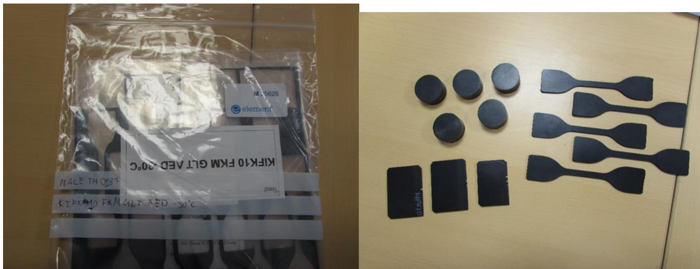
Figure A.1 As received material/before start of immersion: KIFK 10 FKM GLT AED -30°C
