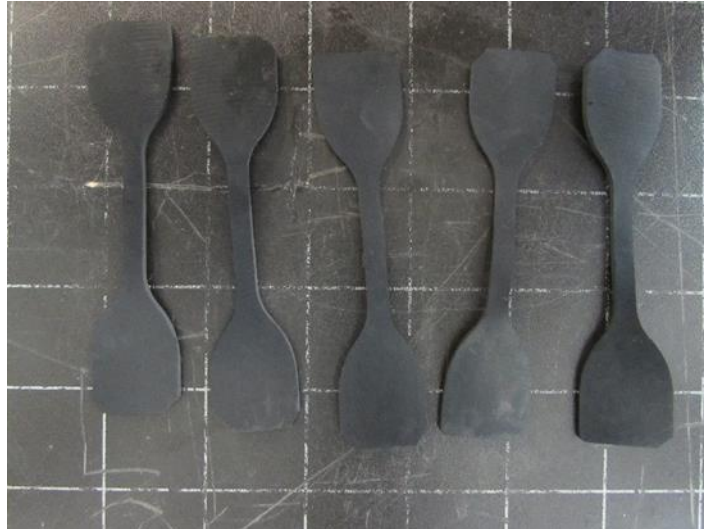
Figure C.1: Tensile dumbbells of - KIFK 10 FKM GLT AED -30°C after immersion
