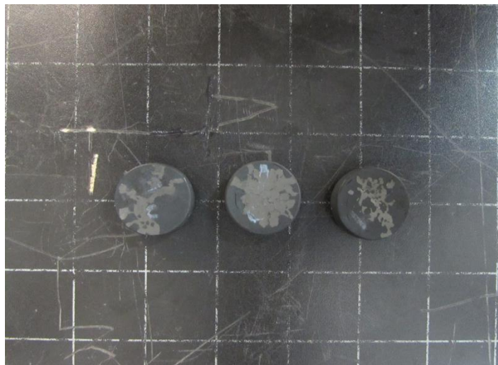
Figure C.3: Compression set button specimens of - KIFK 18 FKMB AED after immersion
