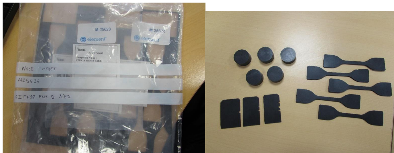
Figure A.1 As received material/before start of immersion: KIFK 18 FKMB AED
