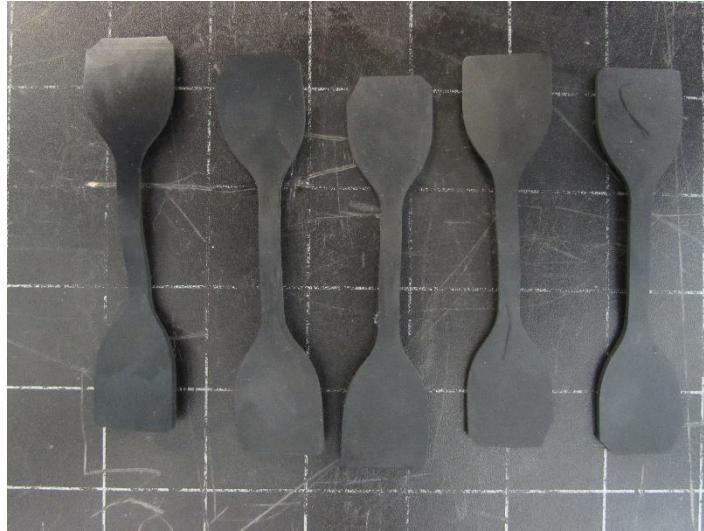
Figure C.1: Tensile dumbbells of - KIFK 18 FKMB AED after immersion
