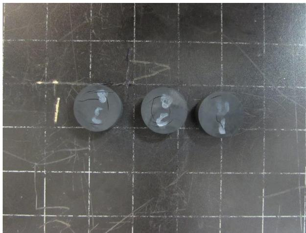
**Figure C.3: Compression set button specimens of - KIFK 15 FKM GLT AE1 AED -46°C, after immersion**
