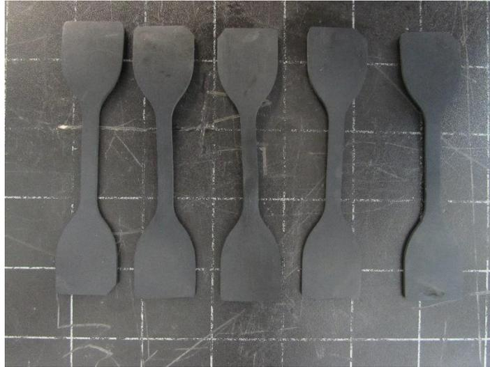
**Figure C.1: Tensile dumbbells of - KIFK 15 FKM GLT AE1 AED -46°C after immersion**
