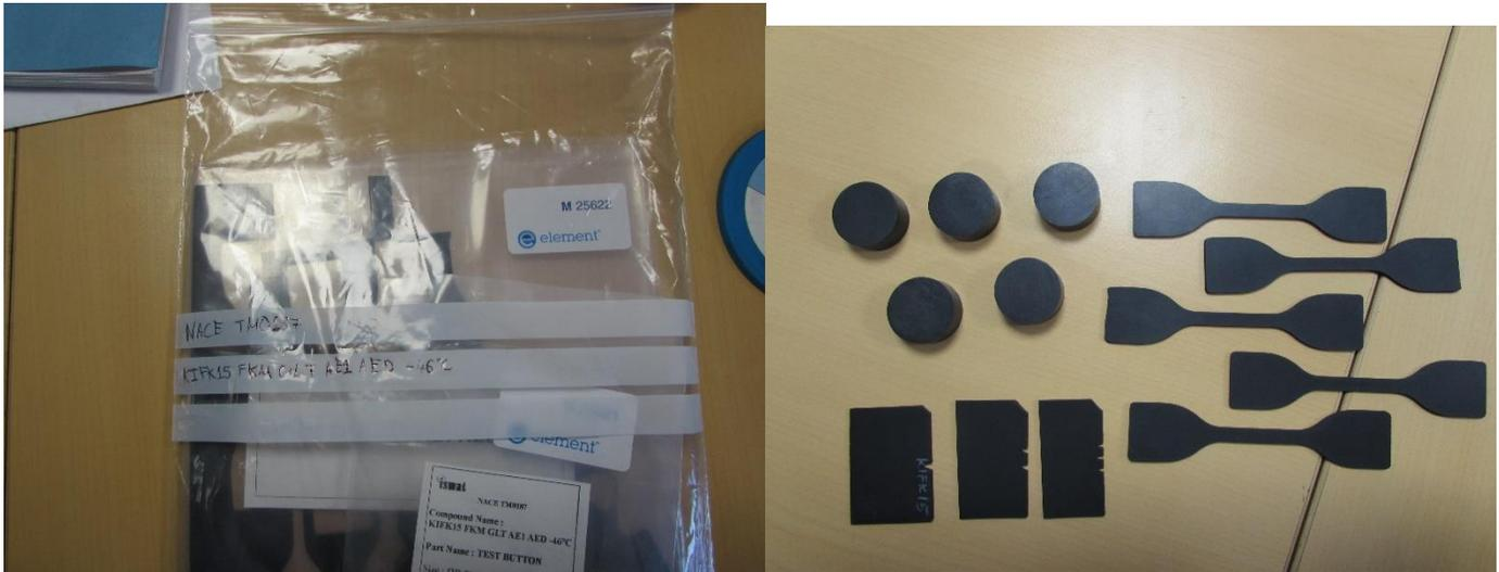
Figure A.1 As received material/before start of immersion: KIFK 15 FKM GLT AE1 AED -46°C
