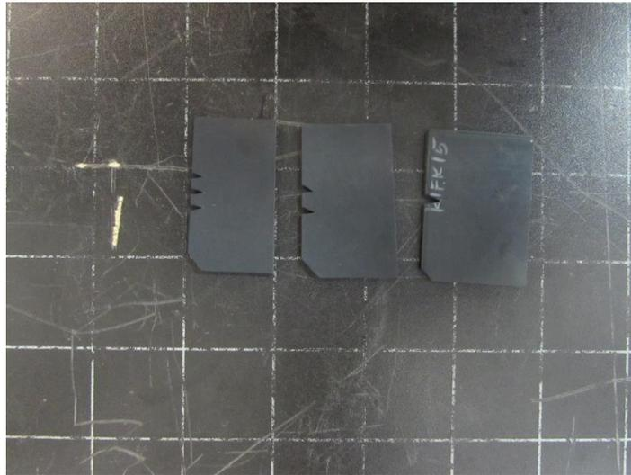
**Figure C.2: MVH specimens of - KIFK 15 FKM GLT AE1 AED -46°C, after immersion**
