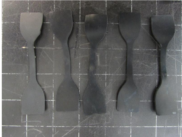
Figure C.1: Tensile dumbbells of - KIFK 11 FKM AED -18°C after immersion
