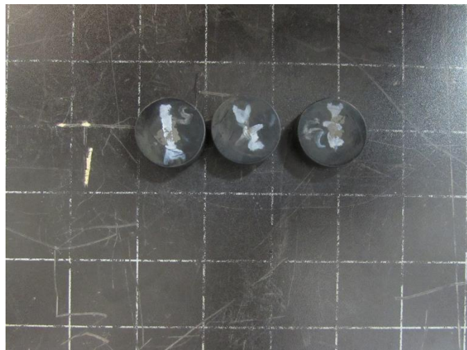
Figure C.3: Compression set button specimens of - KIFK 11 FKM AED -18°C, after immersion
