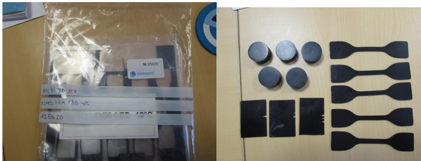
Figure A.1 As received material/before start of immersion: KIFK 11 FKM AED -18°C
